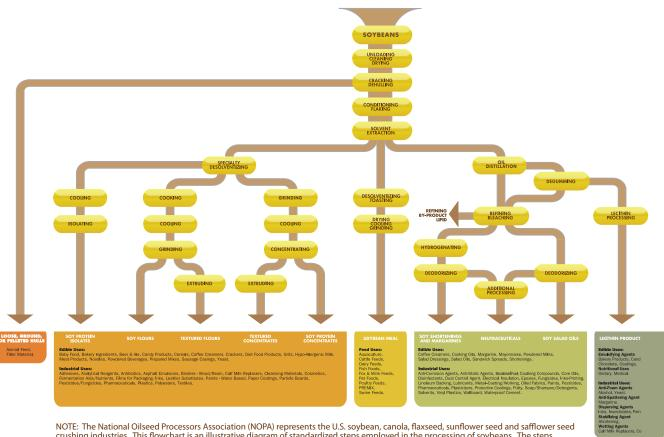
crushing industries. This flowchart is an illustrative diagram of standardized steps employed in the processing of soybeans. The steps employed may vary from plant to plant and from oilseed to oilseed.
